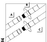
Slide the pair of SLIP SLEEVE (E) until you hear a click to confirm the pair is locked onto the POLE. DO NOT place more than one par on each POLE at a time.
