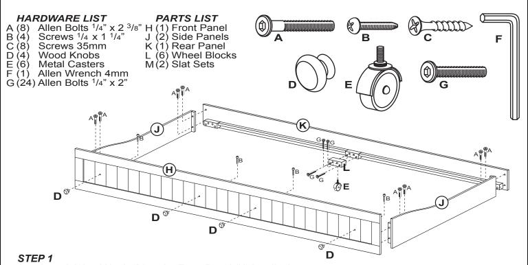
Attach each Wood Knob (D) to the Front Panel (H) by aligning holes and securing from the backside with 1 Screw (B) per each.
