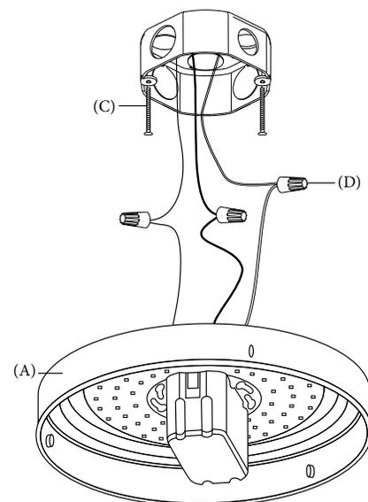
5) Place the LED Fixture Pan (A) over the junction box and onto the Mounting Screws (C) making sure they feed through the Keyhole Slots of the Fixture Pan (A).
