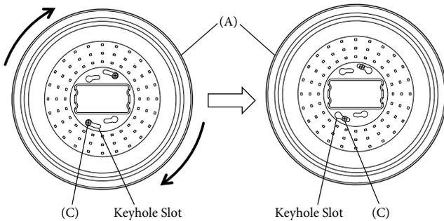
7) Slide the Shade (B) onto the LED Fixture Pan (A) and turn it clockwise until it is secure.
