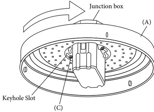
6) Twist the LED Fixture Pan (A) so that Mounting Screws (C) slide into the narrow end of the Keyhole Slots. Tighten the Mounting Screws (C) so that the LED Fixture Pan (A) is flush against the ceiling.
