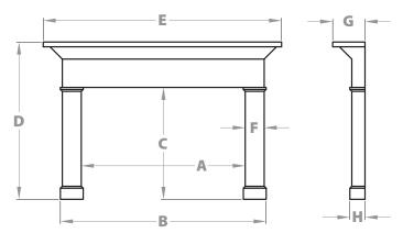
Adjustable filler panels included. Leg Panels: 37-3/8"x 9-3/4" Header Panel: 55-1/4 "x 13-7/8"
