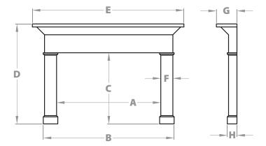
Adjustable filler panels included. Leg Panels: 37-3/8"x9-3/4" Header Panel: 55-1/4"x1 3-7/8"
