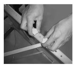
Remove the Lower Leg and then place the Lower Leg back onto the Upper Leg to the desire holes for adjusting the height of the table.
