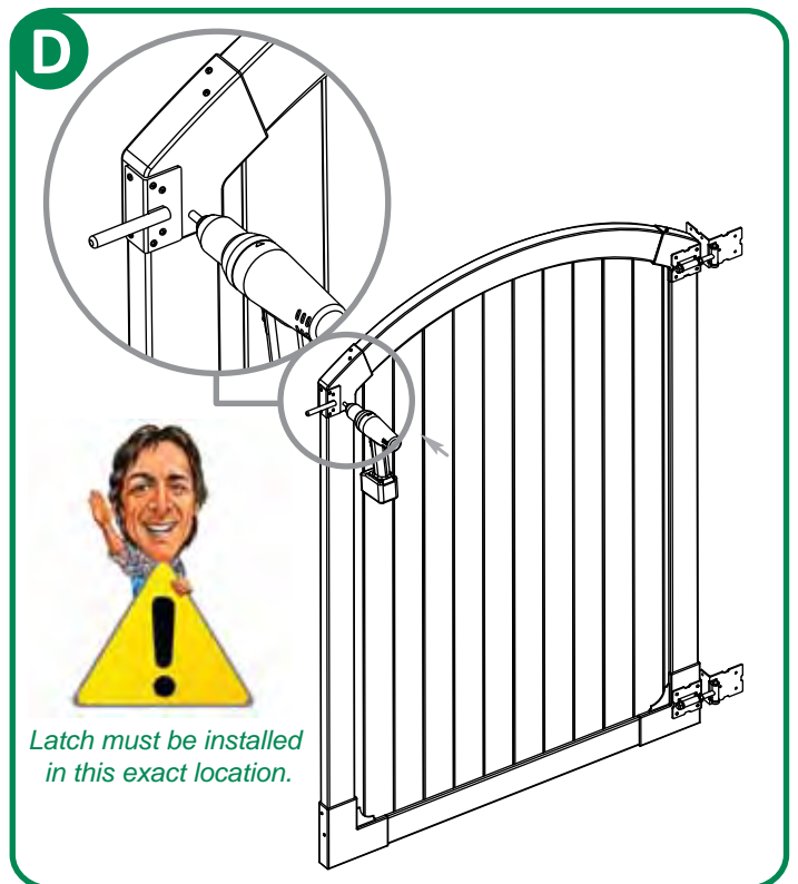
D - Fasten gate latch onto the gate bracket with SHORT screws
