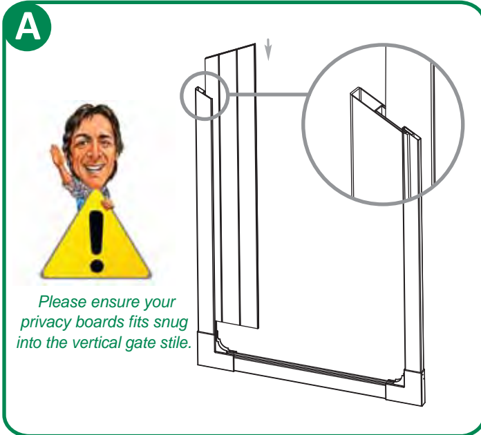
A - Insert tongue and groove privacy board tight into the vertical stile.
