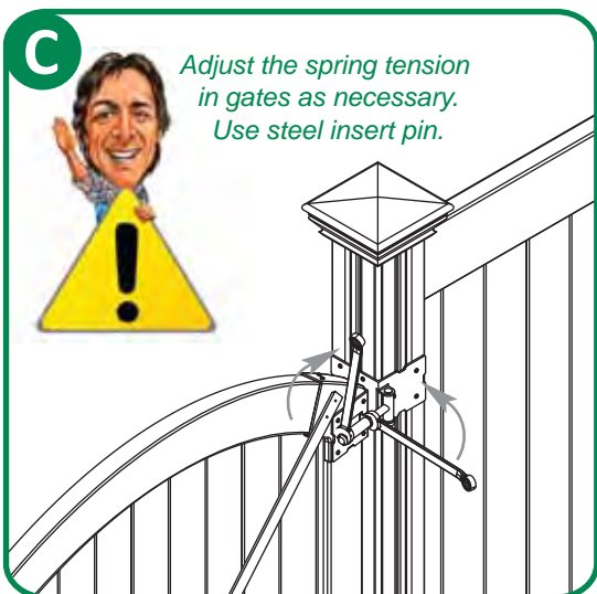
C - Hinges can be adjusted moderately to bring gate into level alignment with post
