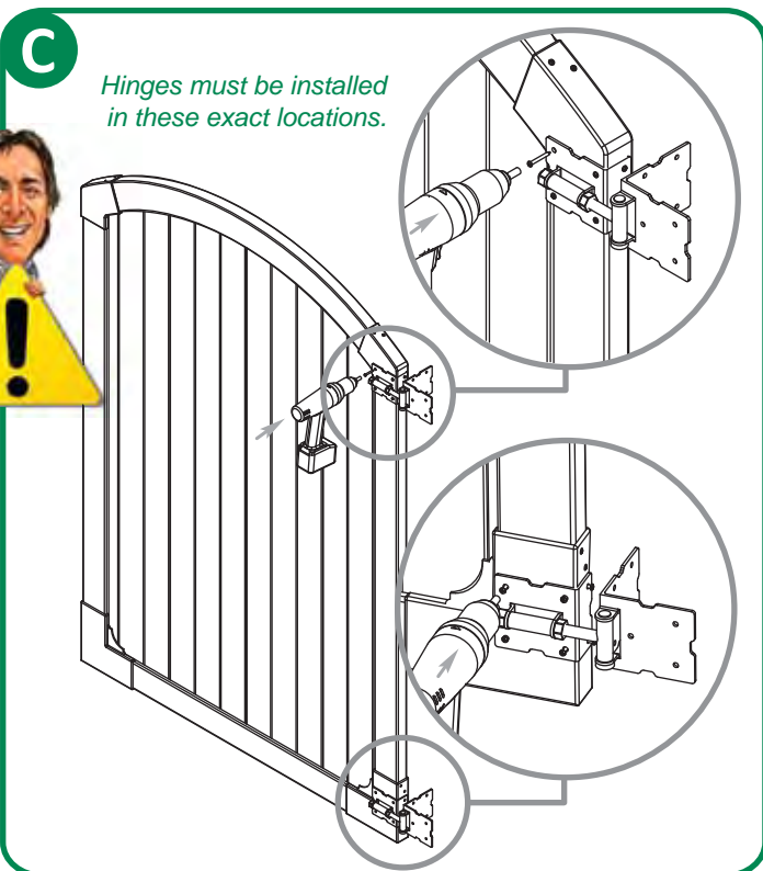
C - Fasten gate hinges onto the gate brackets with SHORT screws
